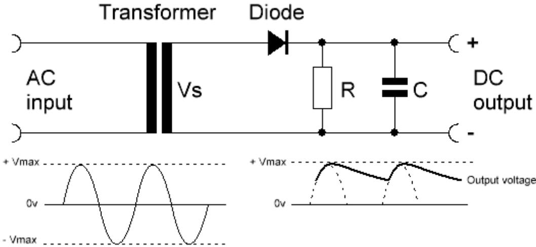
Figure 3. Half-wave rectifier with smoothing capacitor
