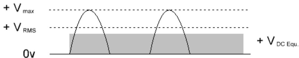
Figure 2. Output DC voltage of the half-wave rectifier
