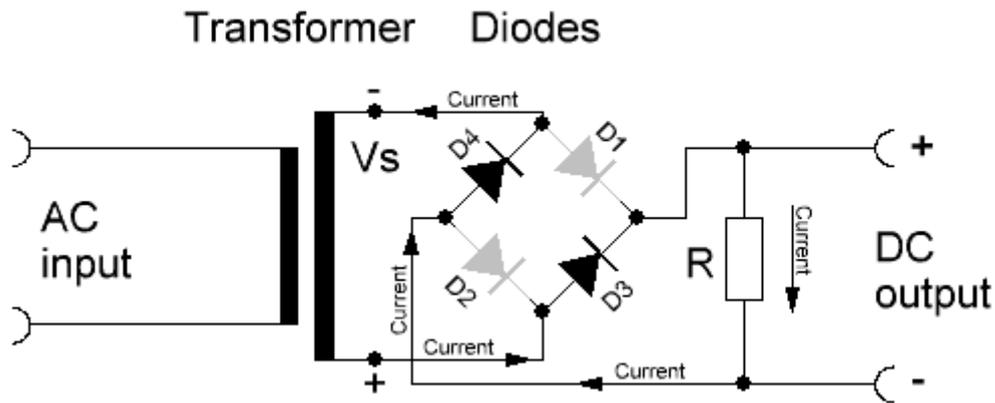
*Figure 7. During negative half-cycle, only diodes D3 and D4 conduct. Diodes D1 and D2 are reverse biased, so they don't conduct.*
