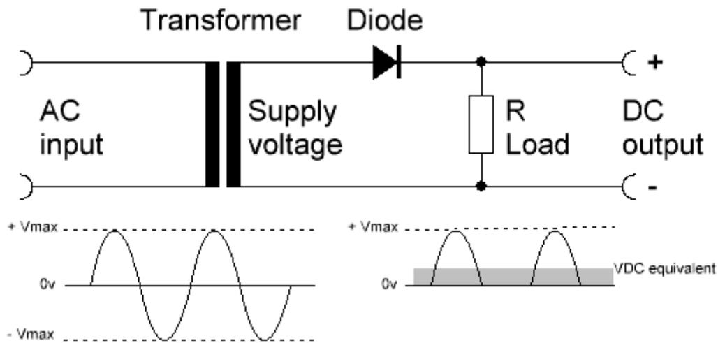
Figure 1. Half-wave rectifier
