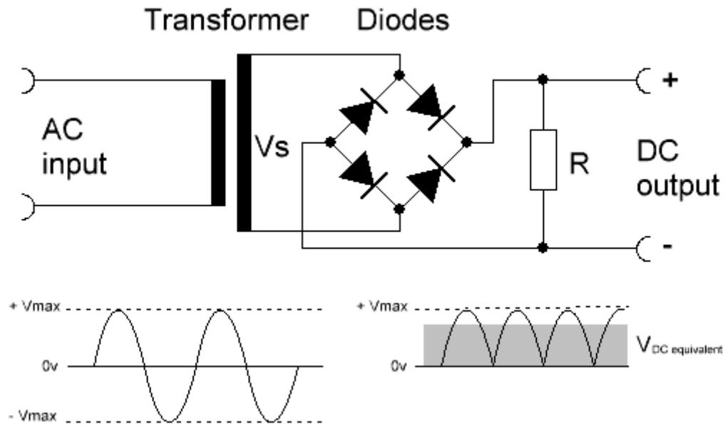
Figure 5. The full-wave bridge rectifier
