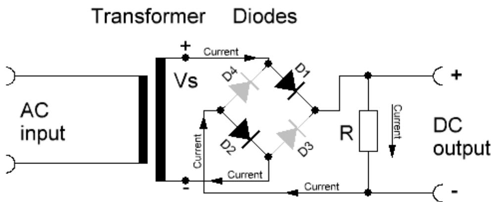
Figure 6. During positive half-cycle, only diodes  $D_1$  and  $D_2$  conduct. Diodes  $D_3$  and  $D_4$  are reverse biased, so they don't conduct.
