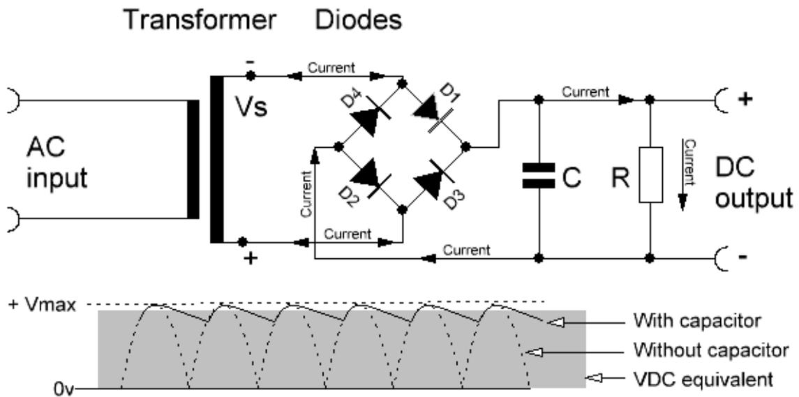
Figure 8. Typical full-wave rectifier with smoothing capacitor
