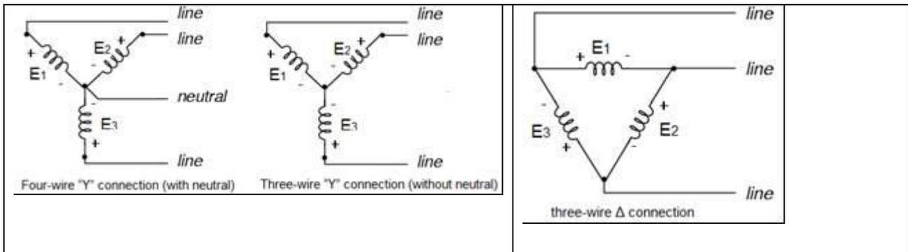
The three-phase systems are classified according to the sets of three electromotive forces (emf) and currents.
