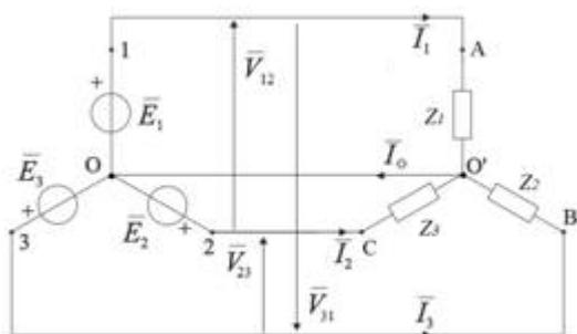
$E_1, E_2, E_3$ : the set of three symmetric voltages
