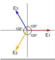
**SYMMETRIC AND BALANCED THREE-PHASE SYSTEMS ( BALANCED WYE-WYE CONNECTION)**
